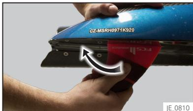
• Then, lower the rear tab into the rear slot of the plug until the mechanism engages the tab.
