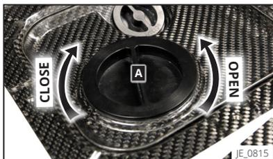
Remove the inspection cover **A** by turning it anticlockwise.
