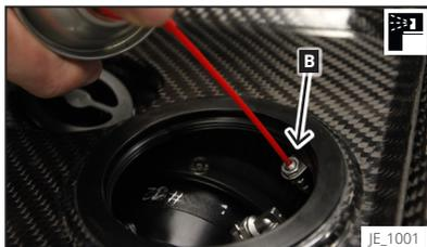
Apply the grease in the opening **B** for 5 seconds.
