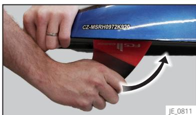
• To remove the fin, grasp the fin and pull upwards.
