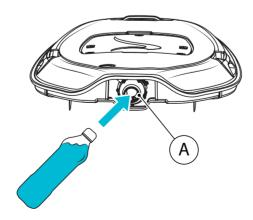
In the battery compartment, put the connector protection in place, and make sure it is tightly sealed around the battery connector.
