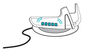
When all LEDs stop flashing the hand control is fully charged.
